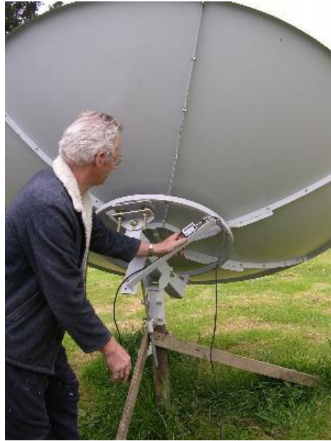
You can see the SF95 satellite finder meter in the picture above, connected via 2m black coax cable. This dish in the picture is a pole mount model but the alignment is done the same.
