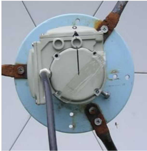
This is the Dual Local Oscillator C Band LNB. This LNB has no markings to indicate skew. Use this picture to help you identify the 'zero' mark. Start with your LNB at this point.
